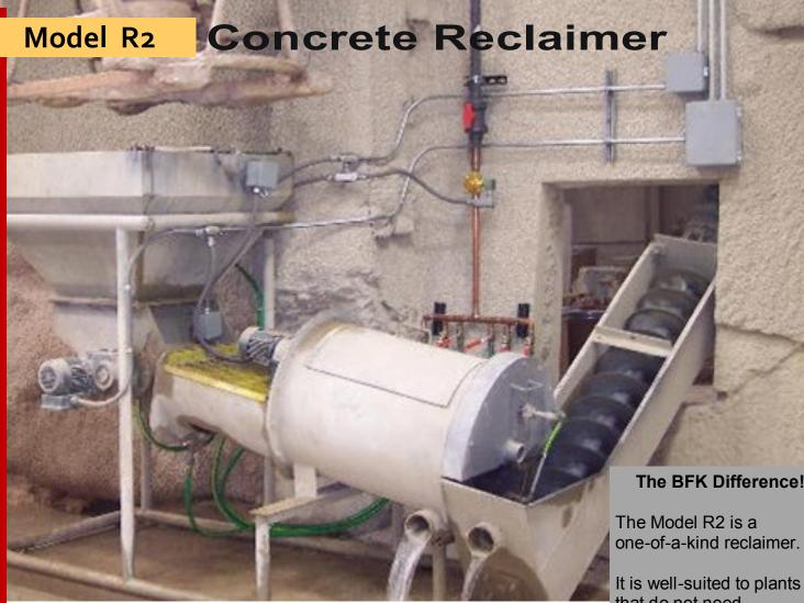
The Model R2 Reclaimer is used where separation of rock and sand is not necessary.
